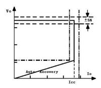
Fig.1. Typical CC/CV Curve
